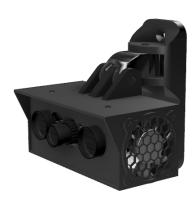
We used a wide-lens IR Camera with IR light attachments to capture high-quality images of bee dances inside the hive. The IR camera is capable of capturing images in low-light conditions, making it suitable for observing bees within the dark environment of the hive. The IR light attachments ensure that the bees are not disturbed by visible light while their dances are being recorded.
